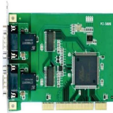
CAN is connected via a 9-pin SUB-D as defined by the CiA DS102-1 standard
