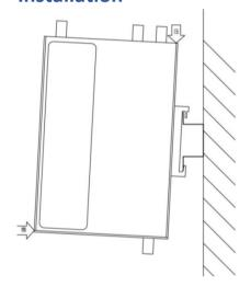
Hang the upper slot on the back of the device into the upper hook of the guide rail, and then press the device down toward the lower hook of the guide rail until it is stuck.
